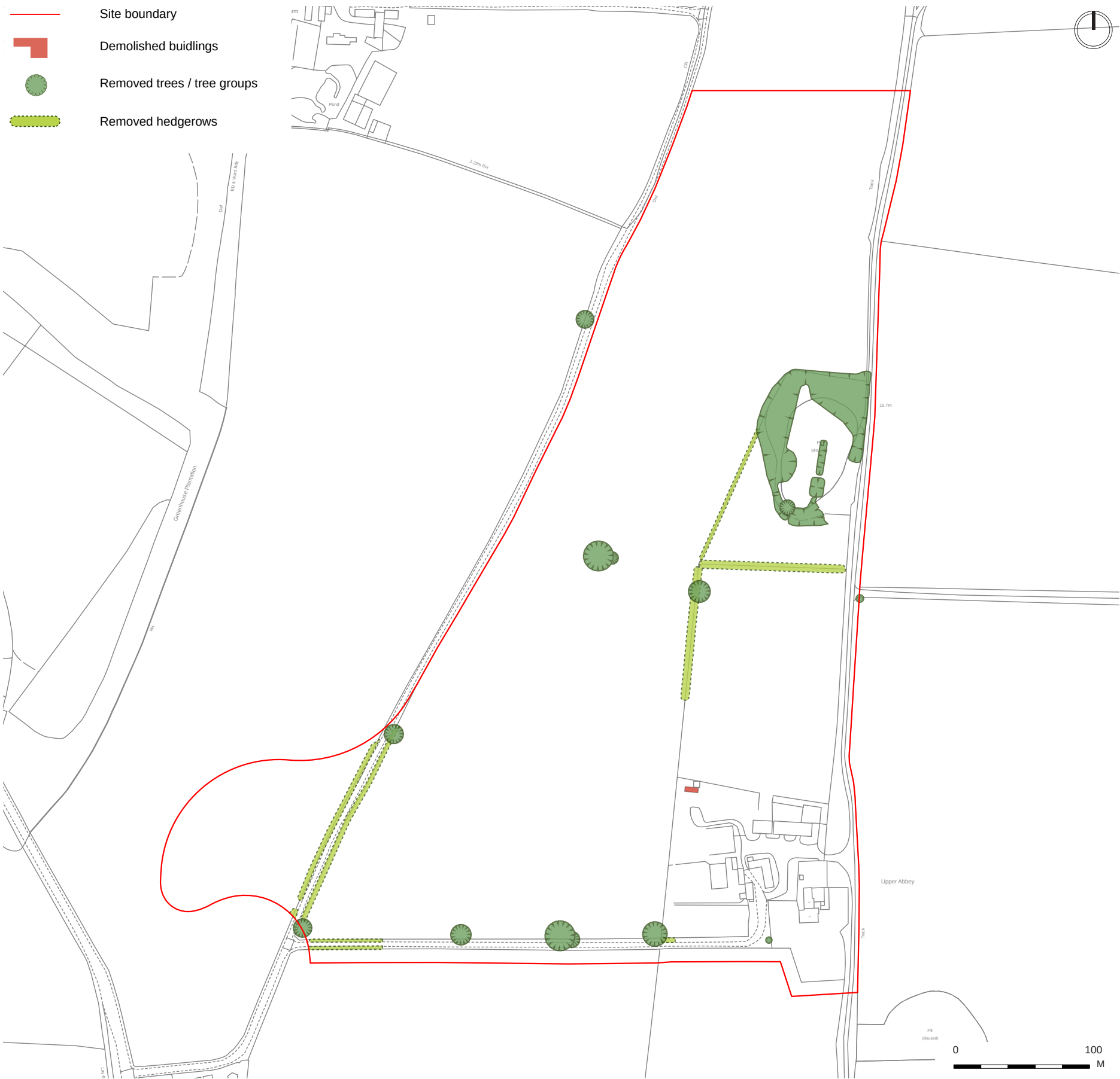
Figure A.57: Clearance and Demolition Plan
